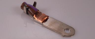
For an optimal process design, a large number of welding parameters must be coordinated in advance. E.g. power, frequency, amplitude, pressure, dwell time, relief, sonotrode shape and geometry and the design of the welding zone. This means that even thin-walled or sensitive components can be welded selectively and with low vibration.
